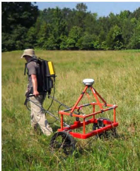
Figure 3-2. EM61-MK2 cart deployed at Camp Butner.
