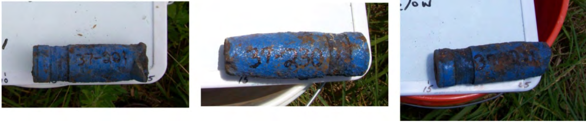
Figure 5-16. Photographs of three 37-mm projectiles without rotating bands seeded at Camp Butner.
