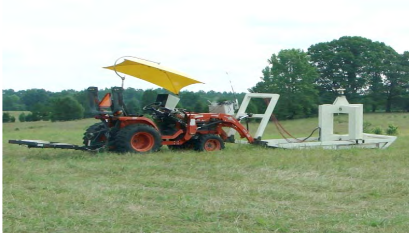
Figure 3-5. MetalMapper configured to collect survey data at Camp Butner.
